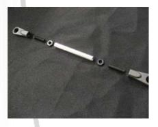
Steering link with necessary parts. Note: measure stock length and add 1.00 inch for proper toe settings.
