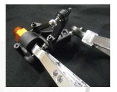
Assembled pic of both upper and lower arms on hub. Notice roll center bushing on upper arm attaching point.
