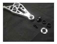
Use these parts to assemble pivot ball socket.
