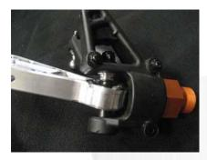
Lower arm installed on hub.
